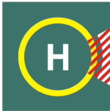
Figure 5-7. Helideck prohibited landing sector marking
